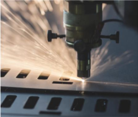
A close-up photograph of a laser cutting machine in operation. A bright orange laser beam is focused on a metal plate, creating a shower of sparks as it cuts through the material. The machine's nozzle is positioned above the plate, and the sparks are being directed downwards.
